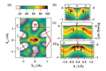
FIG. 1. (Color online) (a) ARPES spectral weight distribution in k space at 300 K integrated at -40 meV over a 20 meV window. Red lines indicate the BZ of the underlying triangular lattice. (b)–(d) Dispersions along the black lines labeled as B, C, and D in (a). The white lines in (b) and (d) are the dispersions calculated in LiVS<sub>2</sub> for  $d_{z^2}$  (solid line) and the two other  $t_{2g}$  (dotted lines: they are degenerate along  $\Gamma$ -M and above  $E_F$  along K-M-K).
