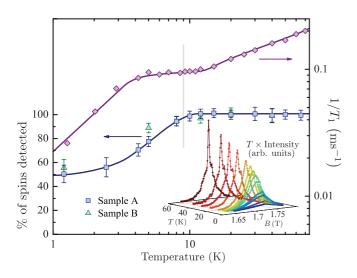
FIG. 4. (Color online) Left-hand axis: Percentage of NMR detectable spins. Right-hand axis: Spin-lattice relaxation rate  $T_1^{-1}$  measured at 72 MHz on sample A. The vertical line indicates the estimated transition temperature. Solid curves are guides to the eye. The 19-MHz spectra with absolute intensity multiplied by T and corrected for  $T_2$  (as much as a 20% correction at high T) are displayed in the inset. The integrated intensity reflects the number of detected nuclei.
