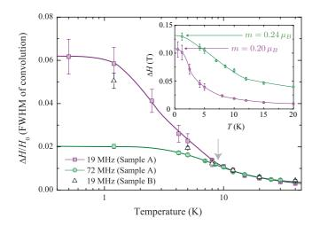
FIG. 3. (Color online) Magnetic broadening  $\Delta H$  for 19 and 72 MHz, scaled by the reference field  $H_0$ . Large error bars at low T result from the proximity of the parasitic phase to the central peak. Sample B, measured at 19 MHz, shows essentially the same result. The inset shows the unscaled  $\Delta H(T)$ , which becomes almost independent of  $H_0$  at low T. Solid lines are guides to the eye.
